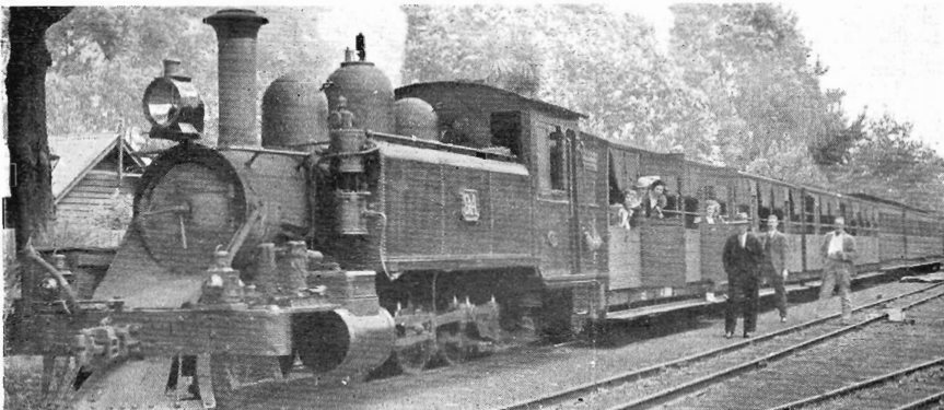
HERE is pictured a passenger train at the Emerald station on the Upper Fern-tree Gully - Gembrook narrow gauge railway. The train is hauled by an 'NA' class, 2-6-2 tank locomotive, No. 9, and consists of a number of open-type excursion vehicles and ordinary compartment cars. (SEE PAGE 3 FOR ARTICLE).
